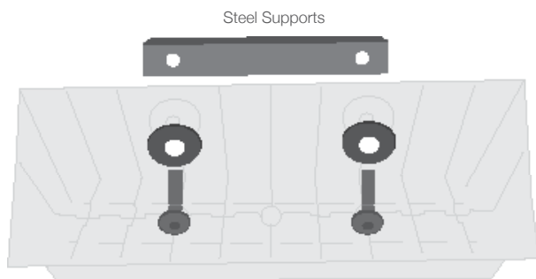
Screws will be used to attach planters into the galvanised steel frame
